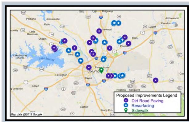
**SCOPE:** The Transportation Improvement Contract 1 includes Resurfacing, Dirt Road Paving and Sidewalk projects. Resurfacing scope: milling, full depth cement stabilization, and/or resurfacing of 23 roads. Sidewalk scope: installation of a 5-foot-wide concrete sidewalk along Capers Avenue. Dirt Roads scope: asphalt paving of 16 dirt roads.
