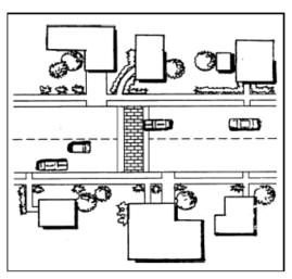
**Speed humps** are rounded raised areas placed across the road. IT E recommends that a speed hump be 12 feet long (in the direction of travel), 3 to 4 inches high, parabolic in shape, and have a design speed of 15 to 20
