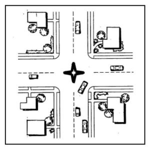
The **star diverter** is a raised island permitting only right turns at an intersection, similar to a forced turn island. They are often compared to the traffic circle (see Speed Control Measures), but are more restrictive. Star diverters are the least common installations among volume control measures.
