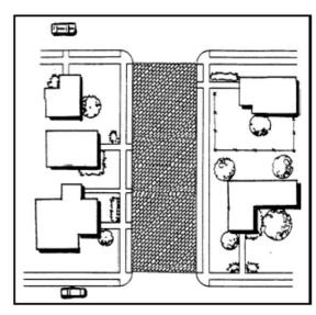
Raised intersections are speed tables covering entire intersections, with ramps on all approaches using brick or other textured materials on the flat section. The textured surface provides a visual cue to the driver to slow down. These intersections rise to sidewalk level, or slightly below to provide a "lip" for the visually impaired. They make entire intersections into pedestrian territory.
