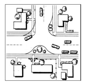
Realigned intersections involve changes to the road alignment that convert T-intersections with straight approaches into curving streets that meet at right angles. A former through movement along the top of the T becomes a turning movement.
