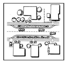
Construction of Chokers is very similar in scope as installation of traffic diverters and neckdowns. In these cases, the redesign must include provisions for curb and gutter, adjustment/installation of catch basins, and landscaping appurtenances.
