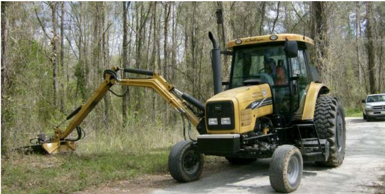
Slope mower cutting County right-of-way
