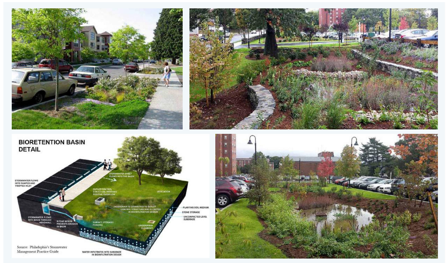
Figure 83: Bioswale Diagram and Examples
