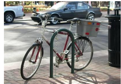
Example of an “Inverted U” bicycle rack. This rack will hold two bikes.
