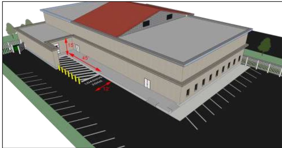
Figure 26-5.2(j): Loading Area Configuration
