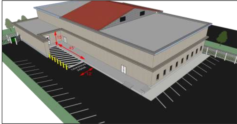
Figure 26-5.2(j): Loading Area Configuration
