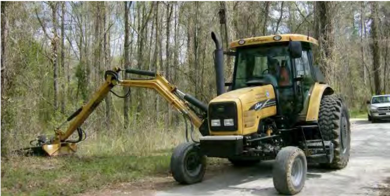
*Slope mower cutting County right-of-way*
