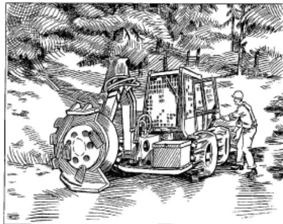
Figure 3. Tractor-mounted mower.
