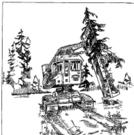
Figure 5. Feller-buncher.
