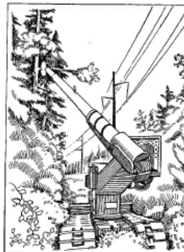
Figure 6. Mechanical pruner.
