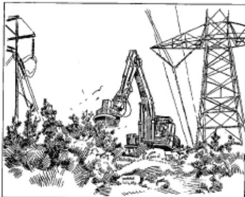
Figure 4. Excavator-mounted mower.
