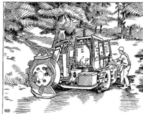
Figure 3. Tractor-mounted mower.
