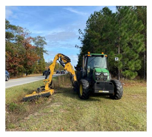
Slope mower cutting County right-of-way
