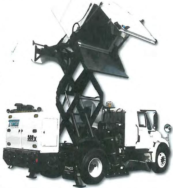
The Model 500x® features a variable dump height from 2 feet to 11 feet from the tip of the discharge chute to the ground with the hopper fully tilted, enabling the 500x® to dump into various size containers. The fast 68 second dump cycle means more time sweeping, less time dumping.
