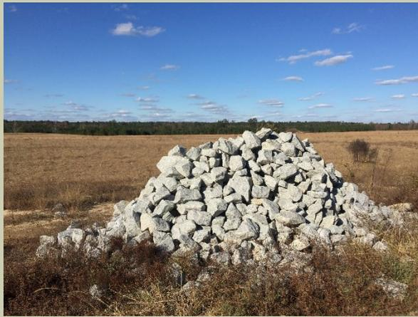
Granite is an igneous rock comprised of the minerals feldspar, quartz, and mica. It is one of the most common rock types on Earth and has a variety of commercial uses, from rip-rap for drainage and slope protection to building stone. Granite is also used for ornamental statues and monuments. Granite is mined throughout SC, and SC's state stone is Winnsboro blue granite. Because granite takes millions of years to form, it is considered a non-renewable natural resource.
